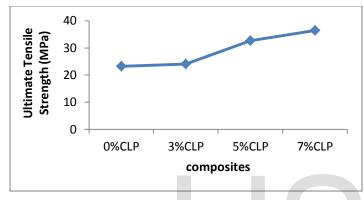
Fig.5. Ultimate tensile strength of the cassava leaves composites
