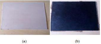
Fig.1. Extruded polypropylene based composites produced for (a) pure polypropylene, (b) Cassava leave powder reinforced with polypropylene.
