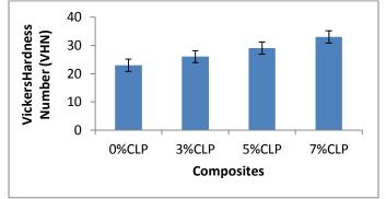
Fig.4. Hardness of the composites
